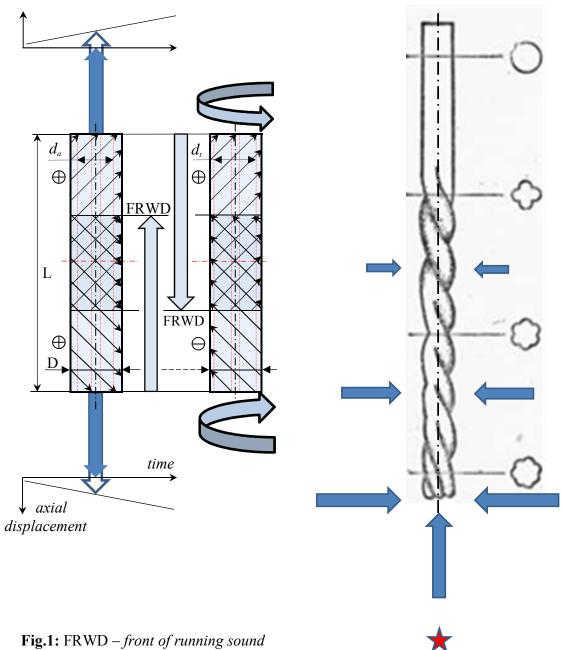
**Fig.1:** FRWD – front of running sound wave of displacement;  $+45^{\circ}$  and  $-45^{\circ}$  are constant angles;  $\bigoplus$  – tension;  $\bigoplus$  – pressing;  $d_a = 0.707D$ ,  $d_t = 0.841D$
